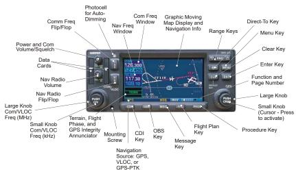
Figure 1 - 430W Series Control and Display Layout
